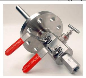
The Oliver Valves D Type Injection Double Block and Bleed Valve features an outlet check valve with two ball pattern primary and secondary isolating valves with a heavy-duty needle vent valve.
